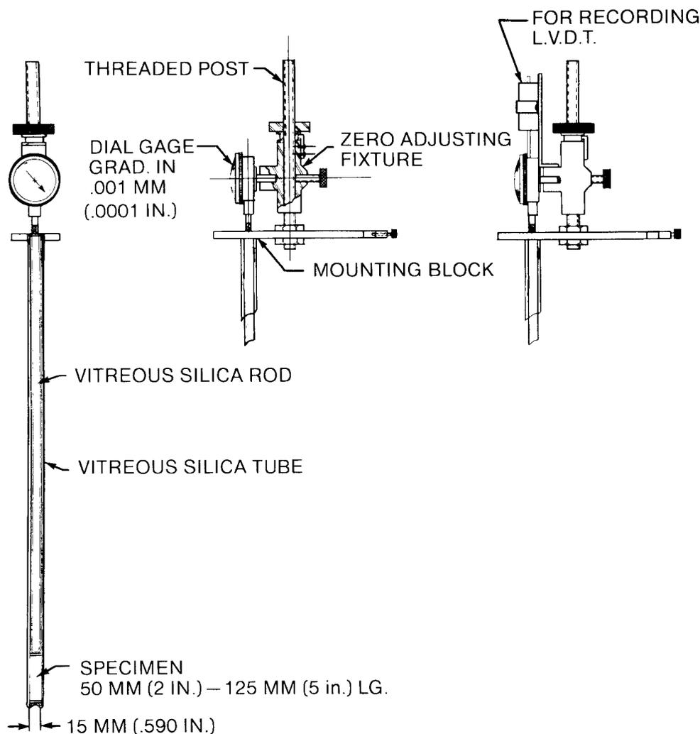
FIG. 1 Quartz-Tube Dilatometer
