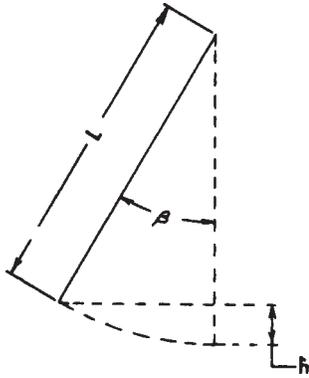
FIG. X3.1 Swing of Pendulum from Its Rest Position
