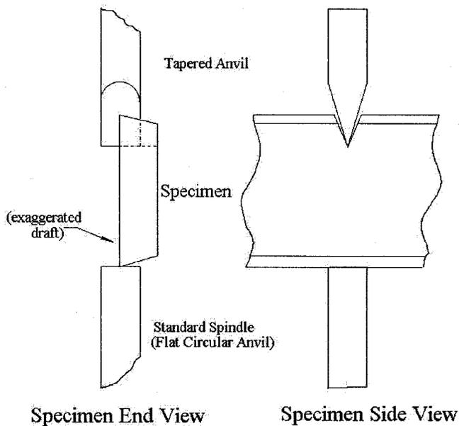
FIG. 5 Notch Depth Measurement on Test Specimens
