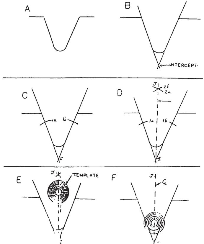
FIG. X1.4 Determining Radius
