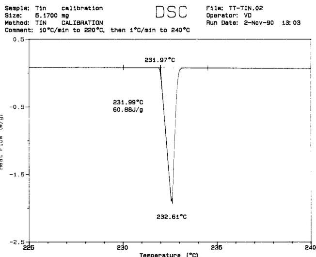
FIG. 1 Indium and Tin Melting Thermal Curves
