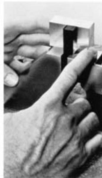
**FIG. 4 Jig for Positioning Specimen for Clamping**
