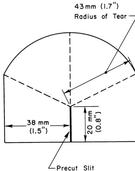
FIG. 1 Constant-Radius Test Specimen for Tear Resistance Test
