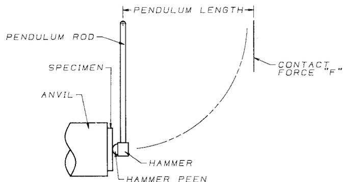
**FIG. 2 Schematic Representation of a Testing Device**
